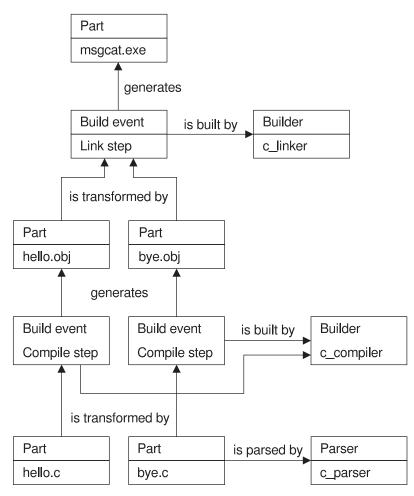
Figure 58. Sample build object model for msgcat.exe
